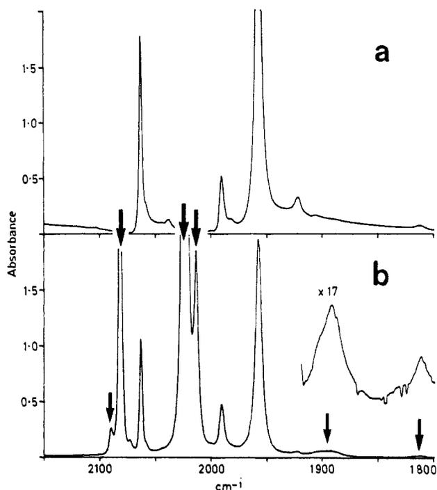
Figure 9. IR spectra showing the synthesis of  $\text{Ru}(\text{CO})_3(\text{H})_2\text{PPh}_3$  by photolysis of  $\text{Ru}(\text{CO})_4\text{PPh}_3$  and  $\text{H}_2$  in *supercritical* Xe at 25 °C: (a) before photolysis; (b) after photolysis. Bands due to  $\text{Ru}(\text{CO})_3(\text{H})_2\text{PPh}_3$  are arrowed; note the lower wavenumber  $\nu(\text{Ru-H})$  region is also shown with an expanded absorbance scale.
