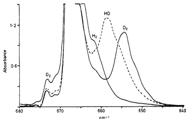
**Figure 3.** IR spectra showing low-frequency bands assigned to Cr(CO)<sub>5</sub>(H<sub>2</sub>), Cr(CO)<sub>5</sub>(HD), and Cr(CO)<sub>5</sub>(D<sub>2</sub>) in liquid Xe at -70 °C. As before, the three traces were recorded in separate experiments. The most intense absorption, which is not labeled, is due to unreacted Cr(CO)<sub>6</sub>.
