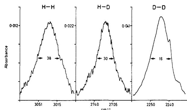
**Figure 2.** IR bands assigned to coordinated  $\text{H}_2$ , HD, and  $\text{D}_2$  in  $\text{Cr}(\text{CO})_5(\text{H}_2)$ ,  $\text{Cr}(\text{CO})_5(\text{HD})$ , and  $\text{Cr}(\text{CO})_5(\text{D}_2)$ , in liquid Xe at  $-70^\circ\text{C}$ . Note that the three bands are observed in separate experiments and are plotted with different absorbance and wavenumber scales. The arrows indicate the relative half-widths of the bands.
