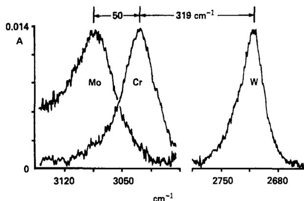
**Figure 1.** IR spectra showing the substantial wavenumber shift between bands assigned to the  $\nu(\text{H-H})$  vibration of coordinated molecular dihydrogen in  $\text{Mo}(\text{CO})_5(\text{H}_2)$ ,  $\text{Cr}(\text{CO})_5(\text{H}_2)$ , and  $\text{W}(\text{CO})_5(\text{H}_2)$  in liquid Xe at  $-70^\circ\text{C}$ . Note that the three traces were recorded in separate experiments and that the absorbance scale refers to the Mo traces.
