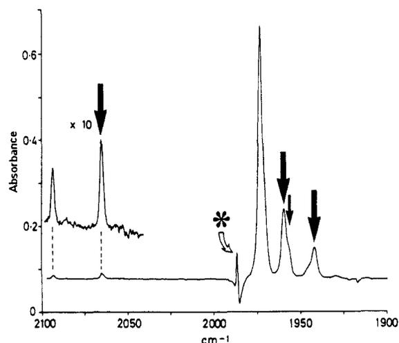
**Figure 4.** IR spectrum in the ν(C-O) region, obtained after photolysis of Cr(CO)<sub>6</sub> and H<sub>2</sub> in liquid Xe at -111 °C. The arrowed bands are assigned to *cis*-Cr(CO)<sub>4</sub>(H<sub>2</sub>)<sub>2</sub> and the unlabeled bands are due to Cr(CO)<sub>5</sub>(H<sub>2</sub>). The asterisk marks the residual feature, left after computer subtraction of the IR band of unphotolyzed Cr(CO)<sub>6</sub>.
