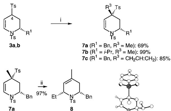
**Scheme 5.** (i) LDA (1.1 eq), THF-TMEDA (10:1, 0.05M), -78°C, 30 min, then add MeI (2.2 eq) or BrCH<sub>2</sub>CH:CH<sub>2</sub> (1.1 eq), -78°C→rt, 1 h; (ii) Et<sub>2</sub>AlCl (1.2 eq), PhMe (0.15M), rt, 1 h
