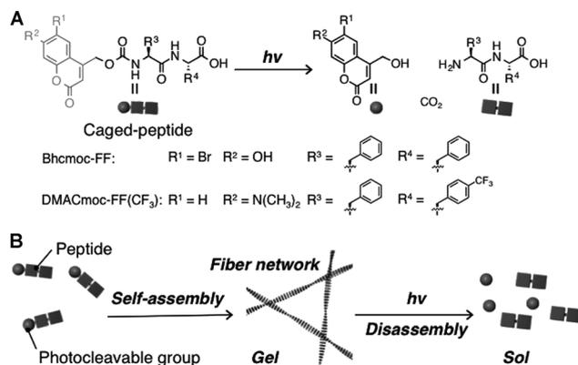
**Figure 1.** A) Photoinduced cleavage of a caged-peptide gelator. B) Schematic representation of the self-assembly of a caged-peptide gelator to form a supramolecular hydrogel and its photoresponsive gel-sol transition.
