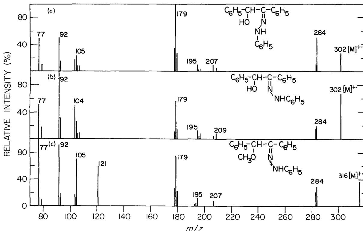
Figure 2. EI mass spectra of (a) *Z*-benzoin phenylhydrazone (**3**), (b) *E*-benzoin phenylhydrazone (**4**) and (c) benzoin methyl ether phenylhydrazone (**13**).
