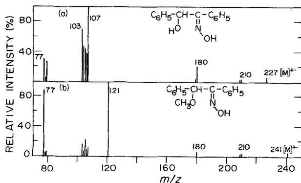
**Figure 1.** EI mass spectra of (a) benzoin oxime (**2**) and (b) benzoin methyl ether oxime (**12**).
