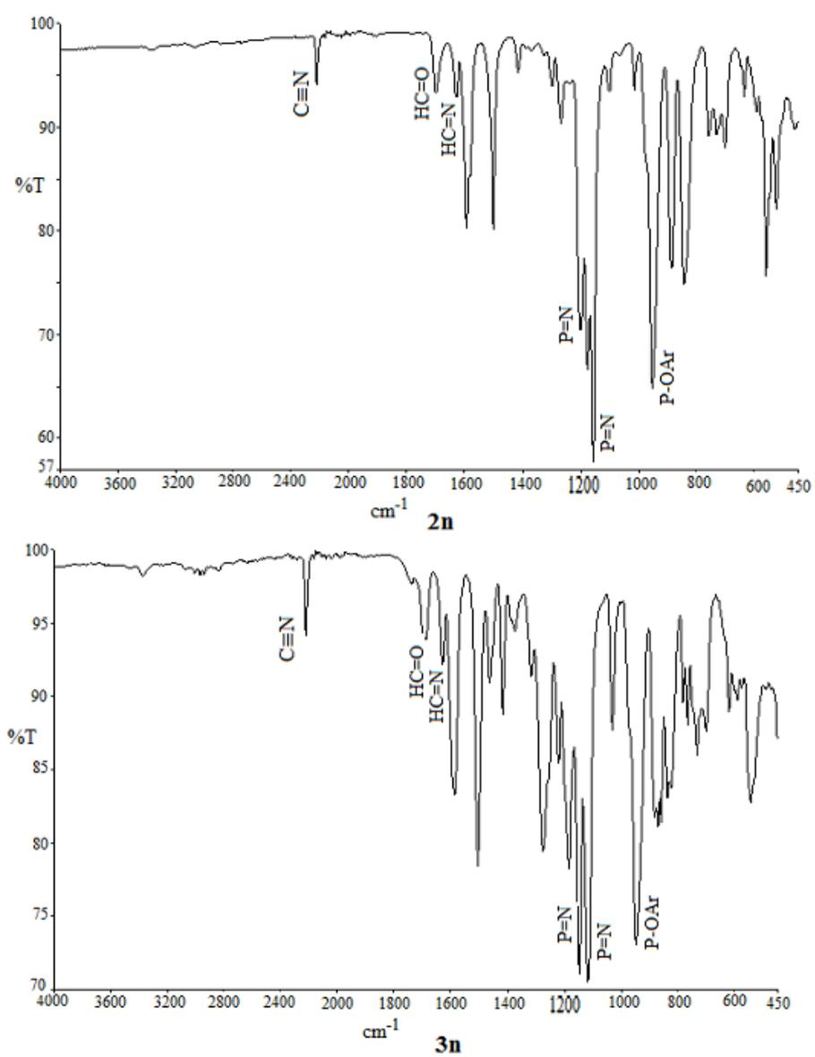
**Fig. 1.** FTIR spectra of the compounds **2n** and **3n**
