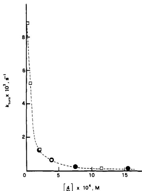
**Figure 4.** Observed "turnover" rate constant,  $k_{\text{turn}}$ , as a function of catalyst **4** concentration (MES buffer, pH = 6.25, [Cu(II)] =  $1.37 \times 10^{-4}$  M); (●) slow process in the cleavage of PNPP; (□) cleavage of **7b**.
