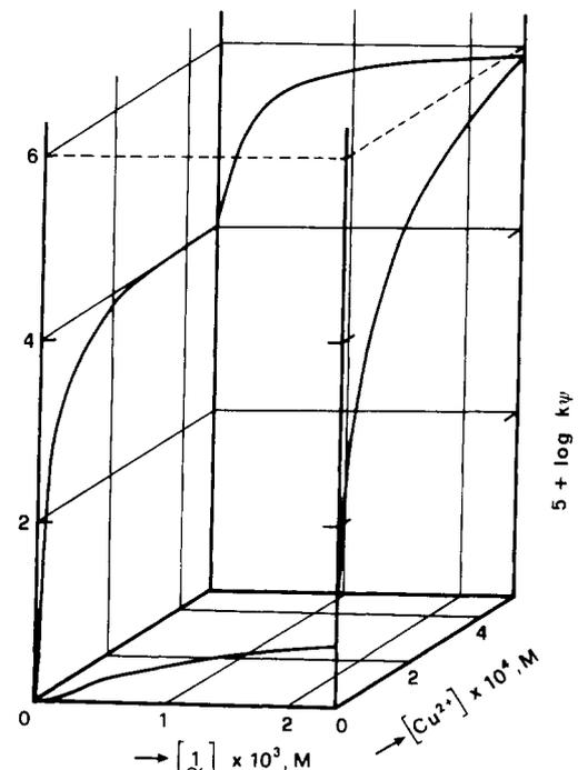
**Figure 2.** Tridimensional representation of the changes of the observed rate constant,  $k_p$ , for the cleavage of PNPP as a function of Cu(II) and catalyst **1** concentrations. (MES buffer, pH = 6.25, 25 °C).
