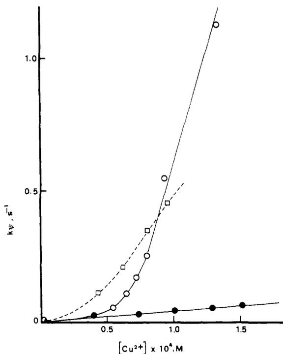
**Figure 3.** Observed rate constant,  $k_{\psi}$ , for the cleavage of PNPP in MES buffer at pH = 6.25 as a function of Cu(II) concentration in the presence of different catalysts at very high [catalyst]/[Cu(II)] ratios: (●) no catalyst added; (○) [1] =  $2.9 \times 10^{-3}$  M; (□), [2] =  $2.9 \times 10^{-3}$  M.
