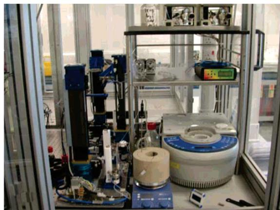
**Figure 4.** Automation of the plug-flow reactor concept. Reagent/product solutions are moved to injection/collection stations by a Kawasaki six-axis robot; reactions are then performed as outlined in Figure 3.
