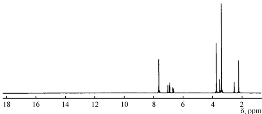
Fig. 3.  $^1\text{H}$  NMR spectrum of Cd(II) complex I.
