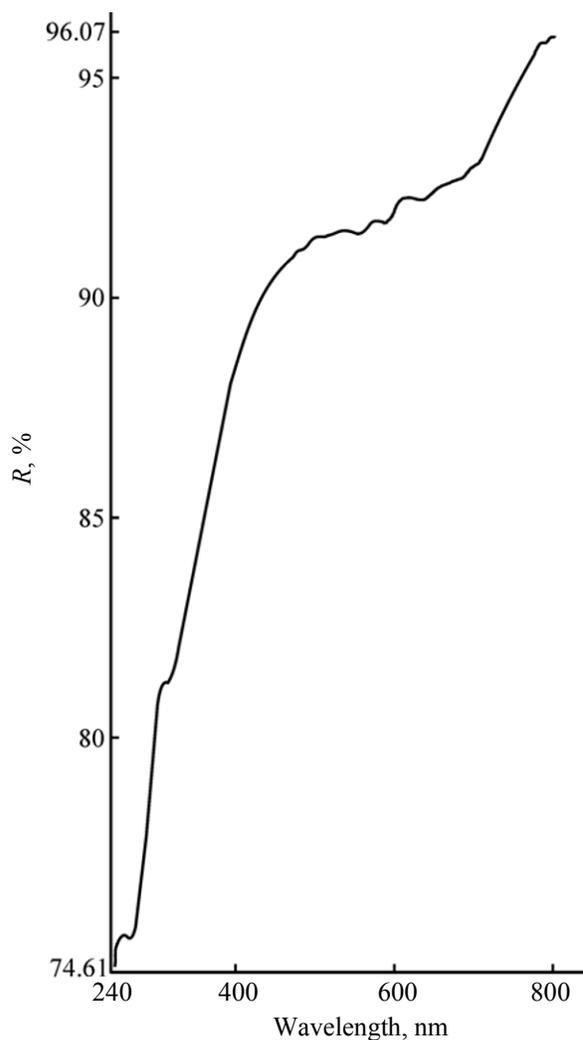
Fig. 5. Solid reflectance spectrum of Ce(III) complex **II**.
