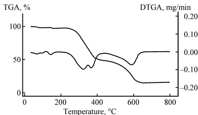
Fig. 7. TG/DTG curve of Cd(II) complex I.
