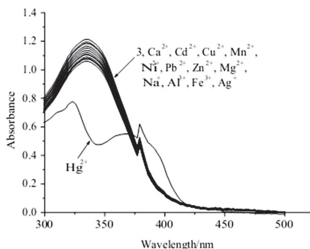
**Fig. 1** UV-Vis spectra of compound **3** (10 μM) upon addition of various ions (20 μM) in DMF and H<sub>2</sub>O (v/v = 1/1).
