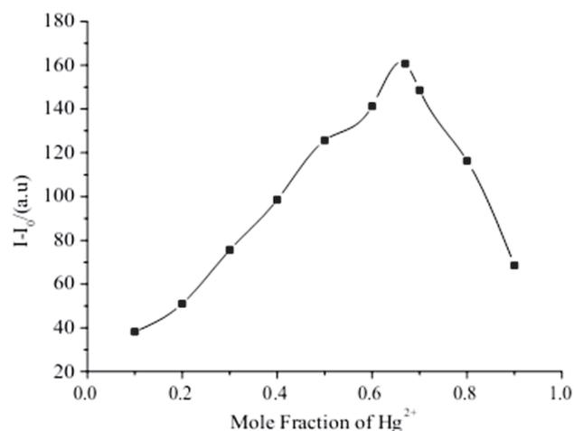
**Fig. 4** Job's plot for determining the stoichiometry of receptor **3** and  $\text{Hg}^{2+}$  ion in DMF and  $\text{H}_2\text{O}$  ( $v/v=1/1$ ),  $I$  and  $I_0$  are the fluorescence intensity of **3** in the presence and absence of  $\text{Hg}^{2+}$ , respectively; the total concentration of **3** and  $\text{Hg}^{2+}$  ion is 0.1 mM ( $\lambda_{\text{ex}}=396$  nm).
