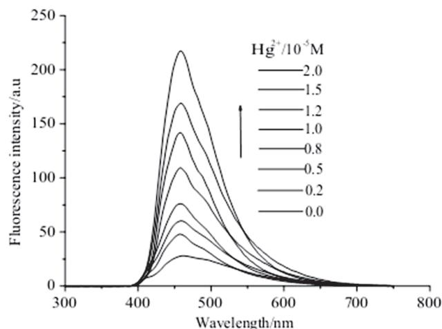
**Fig. 3** Fluorescence emission spectra of compound **3** (10  $\mu\text{M}$ ) for  $\text{Hg}^{2+}$  ion: titration in a mixture of DMF/ $\text{H}_2\text{O}$  ( $v/v=1/1$ ) ( $\lambda_{\text{ex}}=396$  nm).
