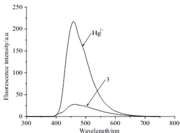
**Fig. 2** Fluorescence emission spectra of compound **3** (10  $\mu\text{M}$ ) upon addition of  $\text{Hg}^{2+}$  and  $\text{Cu}^{2+}$  (20  $\mu\text{M}$ ) in DMF and  $\text{H}_2\text{O}$  ( $v/v=1/1$ ).
