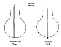
flasks greatly improves this situation, though smooth stirring with normal octagonal stir bars is difficult with these flasks. Although special stir bars have been designed to cope with this problem, it would be more convenient if one could use regular octagonal stir bars.
