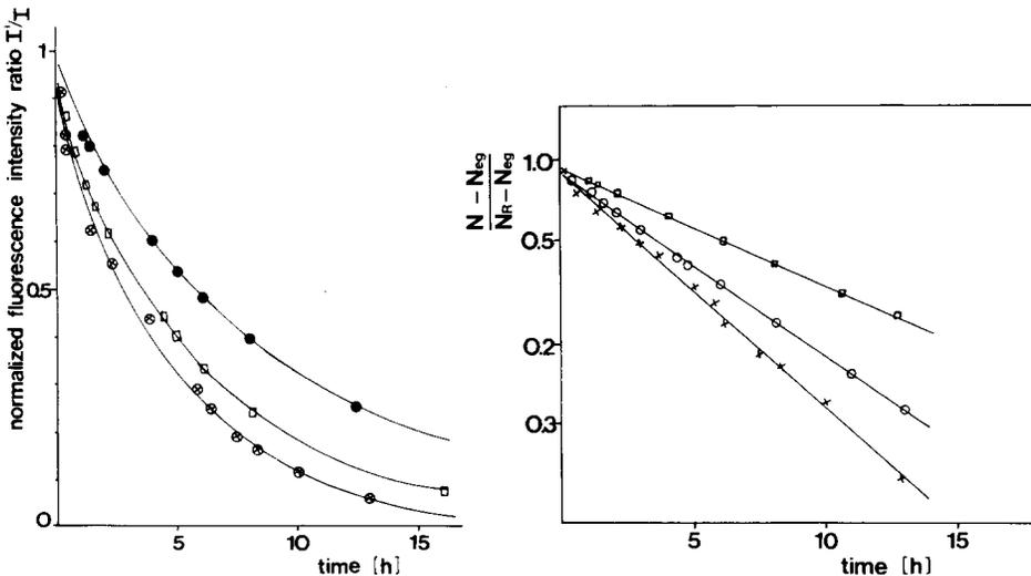
Fig. 5. (a) Time dependence of the normalized fluorescence intensity ratio  $(N - N_{eq})/(N_R - N_{eq})$  for dipalmitoyl lecithin probes containing pyrene lecithin as optical probe. Only the slow exchange process is demonstrated for three different temperatures above the lipid phase transition. Temperature: (●) 314 K; (○) 323 K; (◻) 333 K. (b) The same curves are given in a semi-logarithmic plot. Temperature: (◻) 314 K; (○) 323 K; (×) 333 K.
