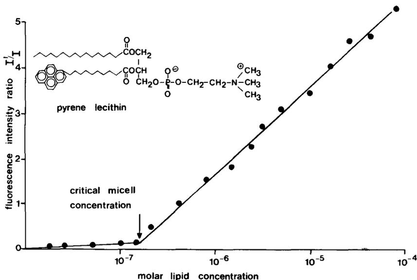
Fig. 1. Fluorescence intensity ratio  $I'/I$  for pure pyrene lecithin vesicles as a function of lipid concentration. The break demonstrates the critical micelle concentration  $c_{CMC} = 1.5 \times 10^{-7}$  M.
