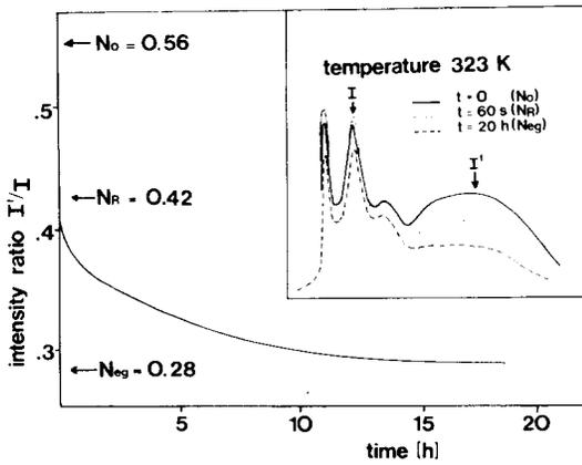
Fig. 4. The fluorescence intensity ratio  $I'/I$  is followed over a time period of approx. 20 h for pyrene lecithin-doped vesicles mixed together with undoped vesicles. The intensity ratio  $N$  decreases from  $N_0$  to  $N_R$  in a rapid exchange process followed by a slow decrease to an equilibrium state  $N_{eq}$ . The insert shows the change in the spectral parameter  $I'/I$  with time.
