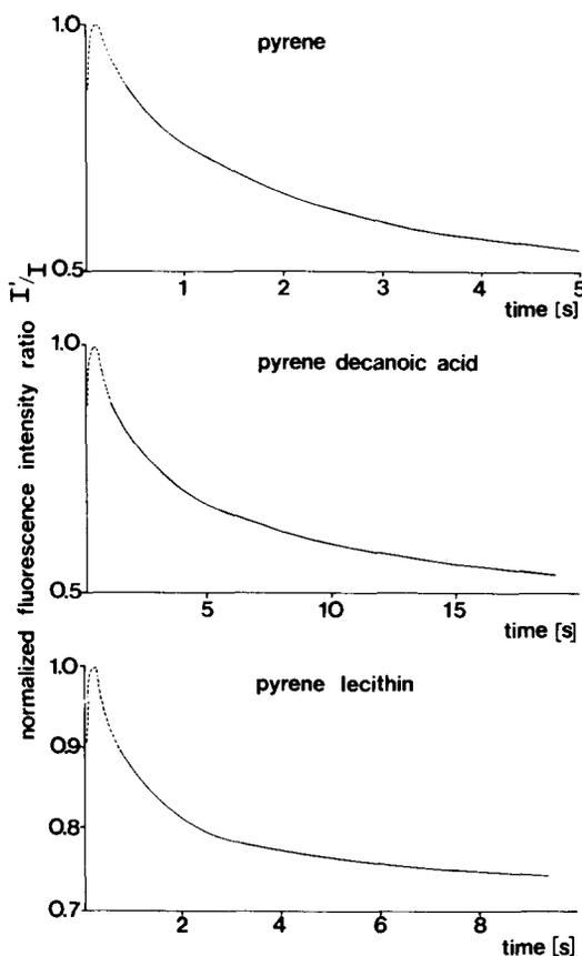
Fig. 2. Time dependence of the intensity ratio  $I'/I$  after rapid mixing in a stopped flow apparatus. Note that  $I'/I$  goes to an equilibrium state in the case of pyrene and pyrene decanoic acid but not in the case of pyrene lecithin. Because of instabilities in the first second after mixing the dotted part is not used to evaluate the exchange constants.
