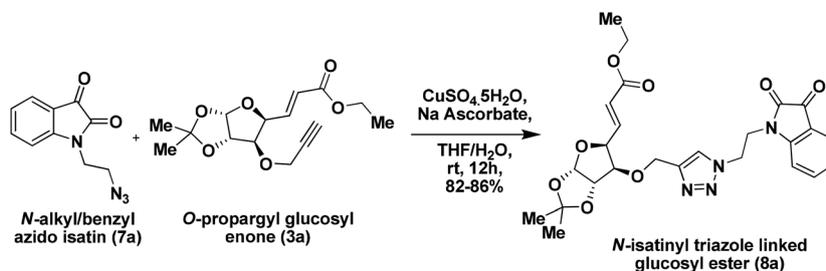
Scheme 4 Model reaction: synthesis of triazole linker 8a.
