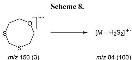
It is known that elimination of  $HS^{\cdot}$  and  $HS_2^{\cdot}$  radicals is characteristic of fragmentation of all 2-aryl-1,3-dithianes [8]. The presence of a heteroaromatic ring in molecules **IIa–IIe** completely suppresses these processes, as well as elimination of  $H_2S_2$ ; however, characteristic is the second series of ions arising from expulsion of the X substituent from the pyrazole ring in ion **H** (Scheme 9, Table 1)
