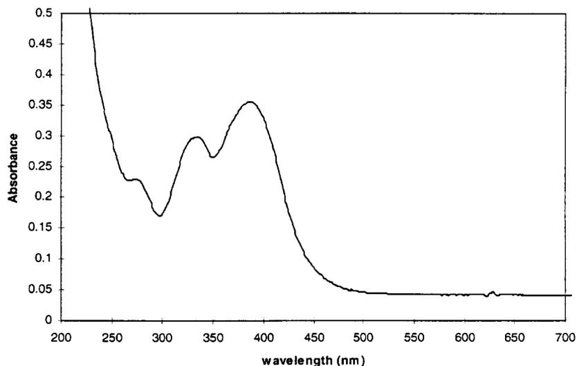
Fig. 6. Electronic absorption spectra of compound I in ethanol solution.
