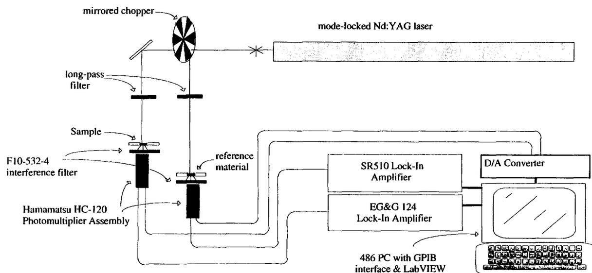
Fig. 1. Experimental configuration for Kurtz powder measurements.
