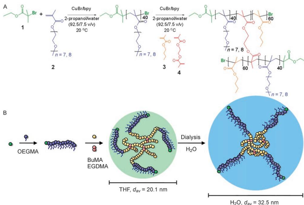
**Figure 1.** A) Synthesis of AB branched block copolymer by ATRP with introduction of the dimethacrylate brancher **4**. B) Schematic of branched copolymer structure in THF and collapse of the poly(*n*BuMA) branched core in water. Diameters refer to z-average values determined by dynamic light scattering. bpy = 2,2'-bipyridine.
