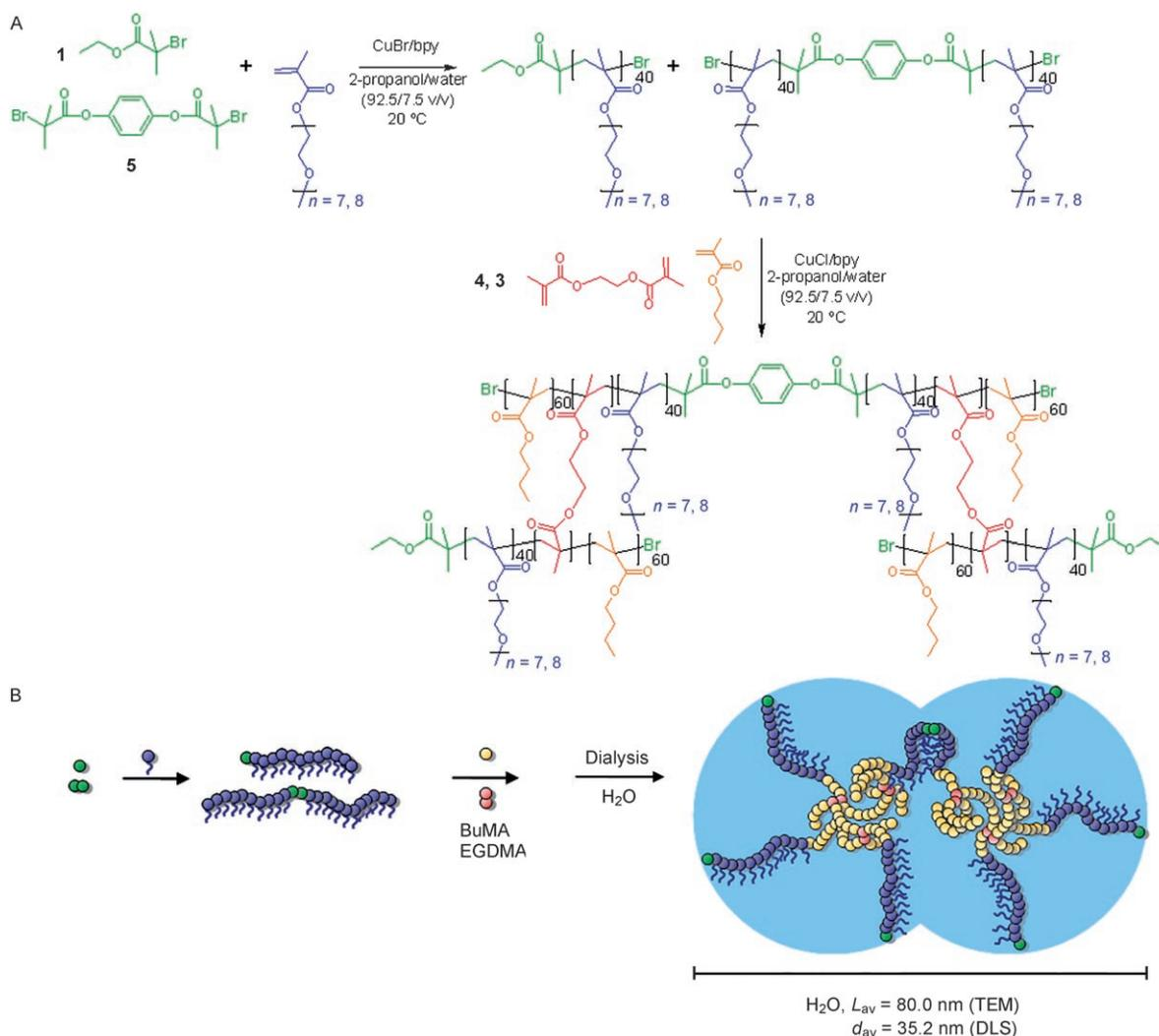
**Figure 3.** A) Targeted synthesis of dumbbell-like polymer nanoparticles by introduction of the difunctional ATRP initiator **5**. B) Schematic representation of a polymer dumbbell nanostructure showing two poly(OEGMA)-protected poly(*n*BuMA) cores covalently connected by a difunctional poly(OEGMA) chain derived from initiator **5**. It should be noted that the DLS diameter is a spherical average and that this is a poor estimate for anisotropic structures.
