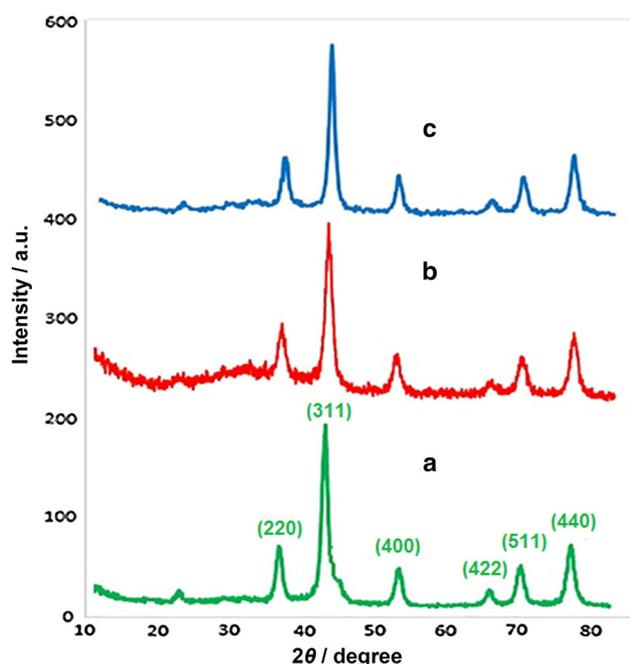
**Fig. 7** The XRD patterns of Fe<sub>3</sub>O<sub>4</sub>-DETA (a), the fresh copper catalyst (b), the recovered copper catalyst after seven times (c)
