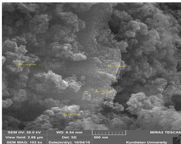
**Fig. 9** SEM image of the recovered catalyst (Fe<sub>3</sub>O<sub>4</sub>-TBA-Br<sub>3</sub>) after seven runs
