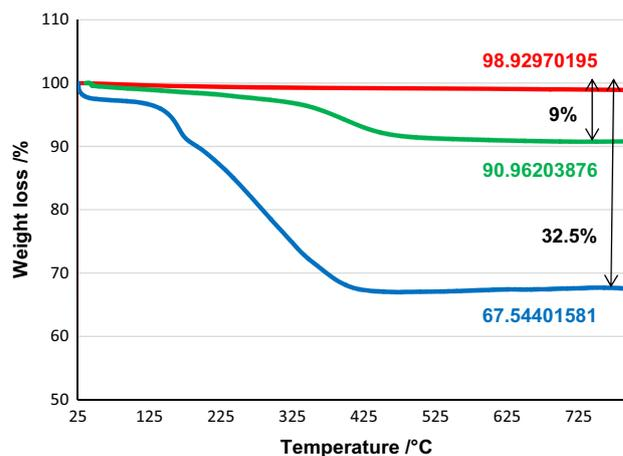
**Fig. 6** TGA curves of  $\text{Fe}_3\text{O}_4$  MNPs (red line),  $\text{Fe}_3\text{O}_4$ -DETA (green line), and  $\text{Fe}_3\text{O}_4$ -DETA-Cu(II) (blue line)
