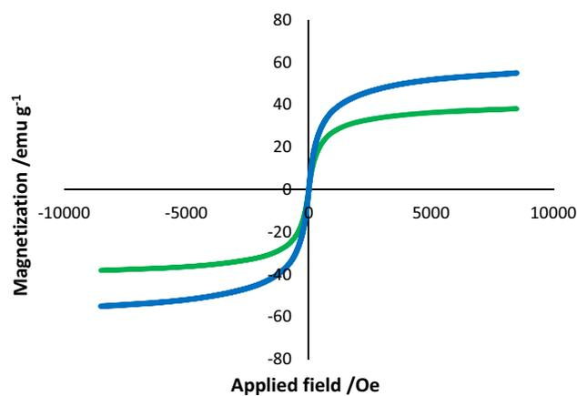
**Fig. 5** Magnetization curves for  $\text{Fe}_3\text{O}_4$  NPs (blue line) and  $\text{Fe}_3\text{O}_4$ -DETA-Cu(II) (green line) at room temperature
