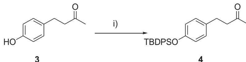
**Scheme 2.** Protection of **3**. (i) TBDPSCl, imidazole, CH<sub>2</sub>Cl<sub>2</sub>, 20 °C, 24 h, 96%.
