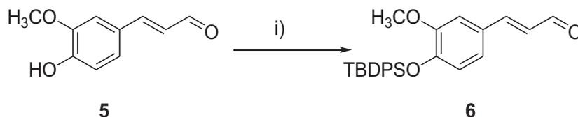
**Scheme 3.** Protection of **5**. (i) TBDPSCl, imidazole, CH<sub>2</sub>Cl<sub>2</sub>, 20 °C, 24 h, 88%.
