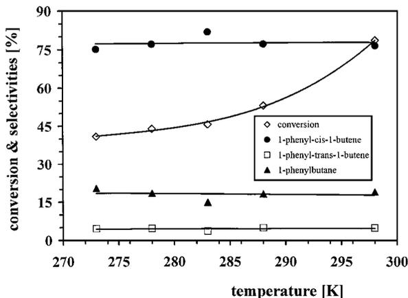
FIG. 5. Transformation of 1-phenyl-1-butyne on Pd-M1 as a function of the reaction temperature. Mass of catalyst, 10 mg;  $p = 10^5$  Pa; reaction time, 60 min; solvent,  $1 \text{ cm}^3$  of *n*-hexane; S : C = 2500.
