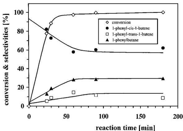
FIG. 4. Transformation of 1-phenyl-1-butyne on Pd-M1 as a function of the reaction time. Mass of catalyst, 10 mg;  $T = 298$  K;  $p = 10^5$  Pa; solvent,  $1 \text{ cm}^3$  of THF; S : C = 2500.
