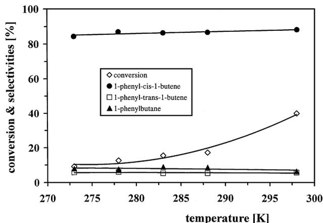
FIG. 7. Transformation of 1-phenyl-1-butyne on Pd-M2 as a function of the reaction temperature. Mass of catalyst, 10 mg;  $p = 10^5$  Pa; reaction time, 60 min; solvent, 1 cm<sup>3</sup> of *n*-hexane; S : C = 2500.
