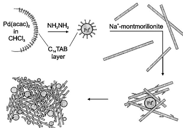
FIG. 1. Schematic illustration of the mechanism suggested for the successive formation of Pd–hydrosol and Pd–montmorillonite in a micellar system.
