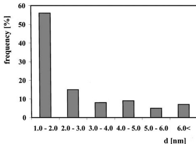
FIG. 3. Particle size distribution obtained for Pd-M2.
