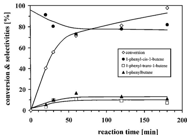
FIG. 6. Transformation of 1-phenyl-1-butyne on Pd-M2 as a function of the reaction time. Mass of catalyst, 10 mg;  $T = 298$  K;  $p = 10^5$  Pa; solvent,  $1 \text{ cm}^3$  of THF; S : C = 2500.
