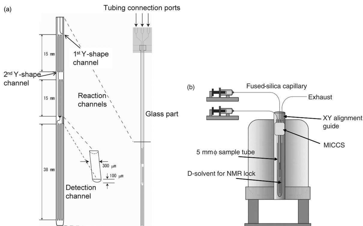
**Figure 1.** (a) The design of flow route of MICCS and (b) the schematic diagram of MICCS-NMR.
