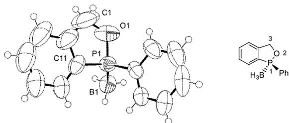
**Figure 2.** ORTEP drawing of *ent*-**2** ( $S_P$ ) derived from (+)-ephedrine at the 50% probability level (one of the two molecules of the unit cell is shown). Selected bond lengths (Å) and angles (deg): P1–B1 1.880(4), P1–O1 1.599(2), O1–C1 1.492(7), B1–P1–O1 115.3(2), B1–P1–C11 114.9(2).
