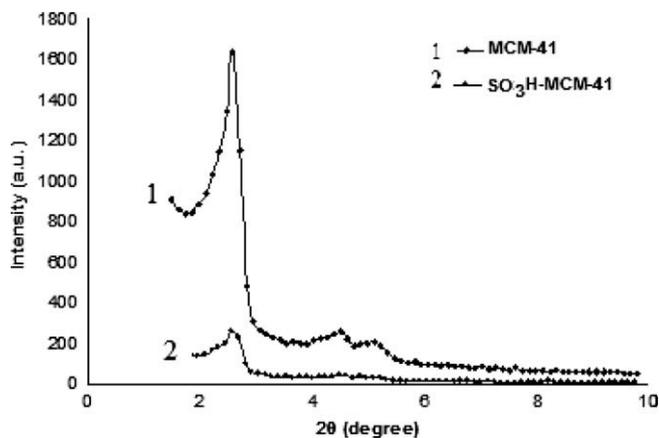
Fig. 1. XRD patterns of MCM-41 and MCM-41-SO<sub>3</sub>H.
