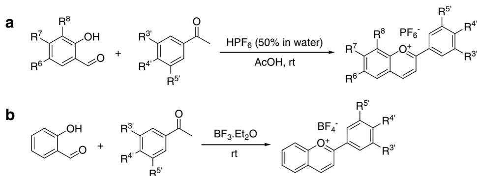
**Scheme 1.** Condensation step for the synthesis of flavylum salts: for (a) A-ring substituted and (b) A-ring unsubstituted derivatives.
