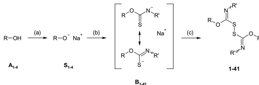
**Scheme 1.** Reagents and conditions: (a) NaH (1 equiv), dry DMF (THF for **3**, **23**, **37**, **38**, **41**), rt, 30 min; (b) R'NCS (**I**<sub>1–38</sub>, 1 equiv), rt, 2 h; (c) TMEDA (2.1 equiv), TsCl (1.6 equiv), rt, 5 h. For the structure list of alcohols **A**<sub>1–4</sub> and isothiocyanates **I**<sub>1–38</sub>, see Figure 4.
