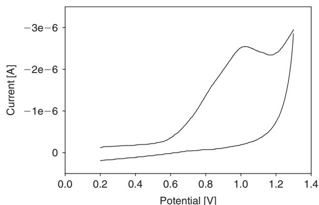
Fig. 3. Cyclic voltammetry of soluble 1,3,4-oxadiazole-pyrazole conjugated polymers **11a**.
