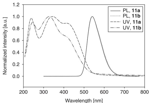
Fig. 2. The UV-vis and PL spectra of **11a** and **11b** in thin film.
