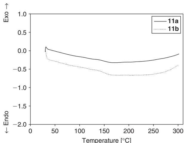
**Fig. 5.** DSC thermograms of soluble 1,3,4-oxadiazole-pyrazole conjugated polymers **11a** and **11b**.
