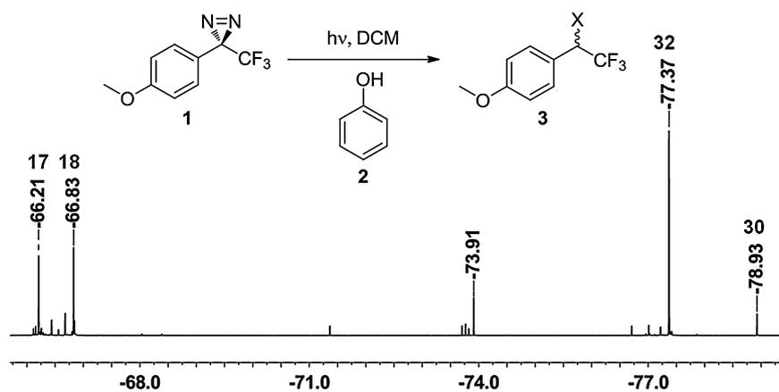
Fig. 1.  $^{19}\text{F}$  NMR spectrum (376 MHz,  $\text{CDCl}_3$ , referenced to  $\text{CFCl}_3$ ,  $\delta_{\text{F}} = 0.0$  ppm) after irradiation (350 nm) of diazirene **1** in the presence of phenol (**2**).
