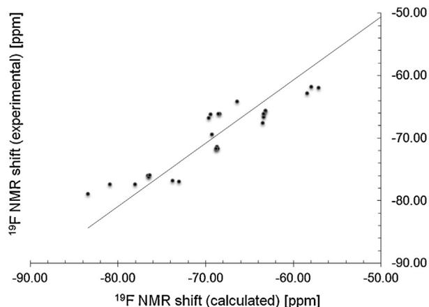
**Fig. 6.** Experimental  $^{19}\text{F}$  NMR chemical shifts of 30 trifluoromethyl compounds (structures see Fig. 2) plotted against the calculated values (standard deviation 2.9 ppm).
