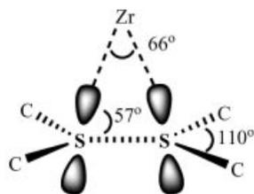
Figure 2. Suggested S–S ( $\sigma$ - $\pi$ )-( $\pi$ - $\pi$ ) interaction in **5** (for clarity, only the filled p orbital on each S atom is indicated); the dashed lines represent the Zr–S vector on the  $C_{2v}$  plane of each binaphthol ligand and the S–S interaction
