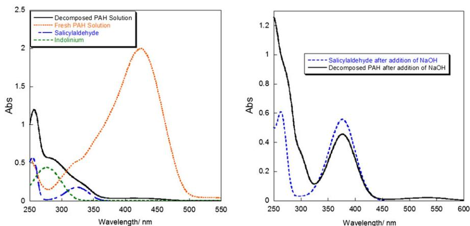
**FIGURE 3** UV-Vis spectra of freshly prepared and decomposed solution of PAH1 compared to that of salicylaldehyde and the indolinium (left), and the spectra of the decomposed solution after addition of a drop of NaOH solution and that of a salicylaldehyde solution after addition of a drop of NaOH solution
