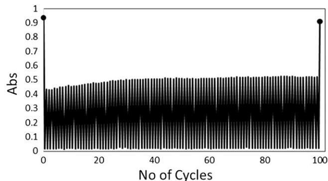
**FIGURE 6** Absorbance of a PAH1 solution at 424 nm during 100 cycles of 1 min irradiation (lower points) followed by 2 min in the dark (upper points)
