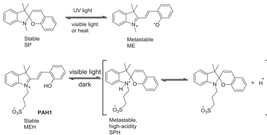
**FIGURE 1** Photoreactions of a common spiropyran (top) and a merocyanine-type photoacid (bottom). ME indicates merocyanine; MEH, protonated merocyanine; SP, spiropyran; SPH, protonated spiropyran; UV, ultraviolet
