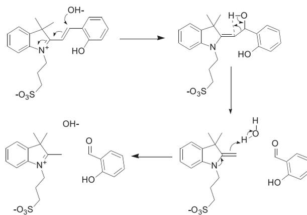
**FIGURE 5** Proposed mechanism of the hydrolysis of a merocyanine-type photoacid
