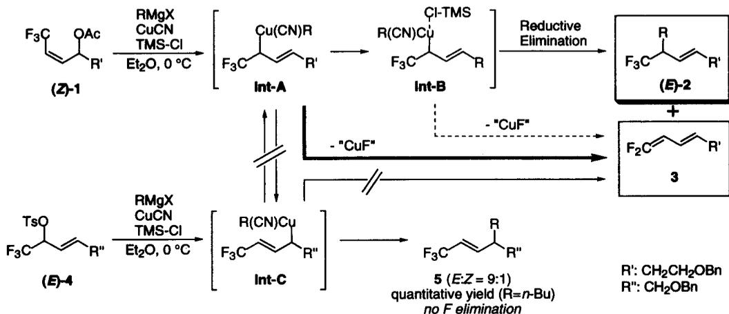
Fig. 2 Reaction Mechanism of the Present  $\text{S}_{\text{N}}2'$  Process
