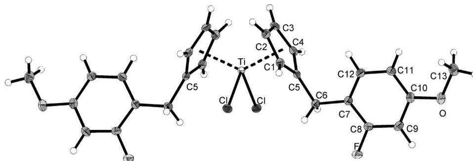
Figure 4. X-ray diffraction structure of bis[(2-fluoro-4-methoxybenzyl)cyclopentadienyl]titanium(IV) dichloride (**3a**); thermal ellipsoids are drawn at the 50% probability level.
