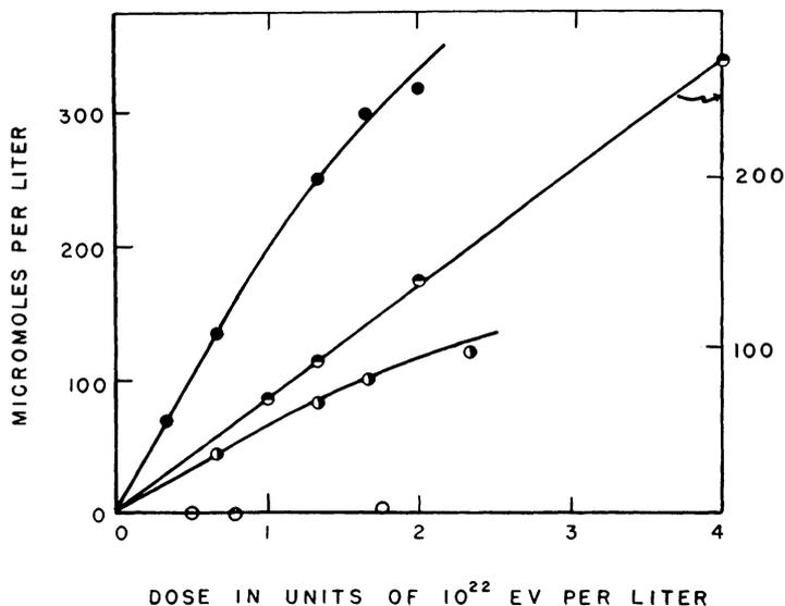
FIG. 1. Radiolysis as a function of dose in air-free neutral solutions of benzene in water. Dose rate:  $4.33 \times 10^{19}$  ev/liter-min. for  $\text{H}_2\text{O}_2$ ;  $5.48 \times 10^{19}$  ev/liter-min. for others. Legend: left ordinate scale: ●  $\text{Ph}_2$ ; ●  $\text{PhOH}$ ; ○  $\text{H}_2\text{O}_2$ ; right ordinate scale: ○  $\text{H}_2$ . Yields:  $G_0(\text{H}_2\text{O}_2) = 0$ ;  $G_0(\text{H}_2) = 0.42$ ;  $G_0(\text{PhOH}) = 0.36$ ;  $G_0(\text{Ph}_2) = 1.22$ .
