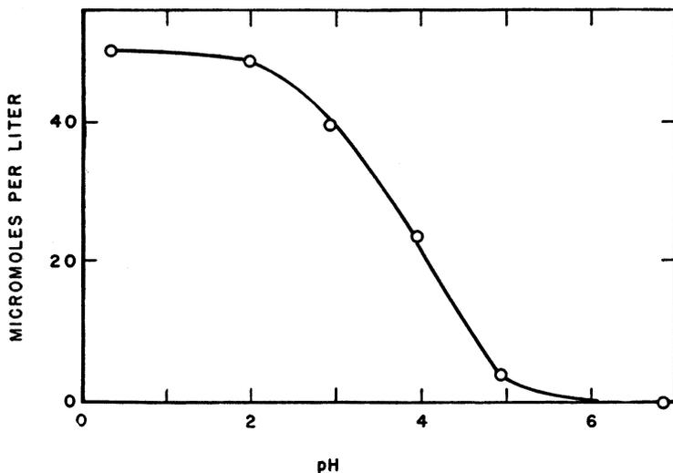
FIG. 3. Production of  $\text{H}_2\text{O}_2$  as a function of pH in radiolysis of air-free solutions of benzene in water:  $\text{H}_2\text{O}_2$  concentrations after 120-minute irradiation. Dose rate:  $4.33 \times 10^{19}$  ev/liter-min.
