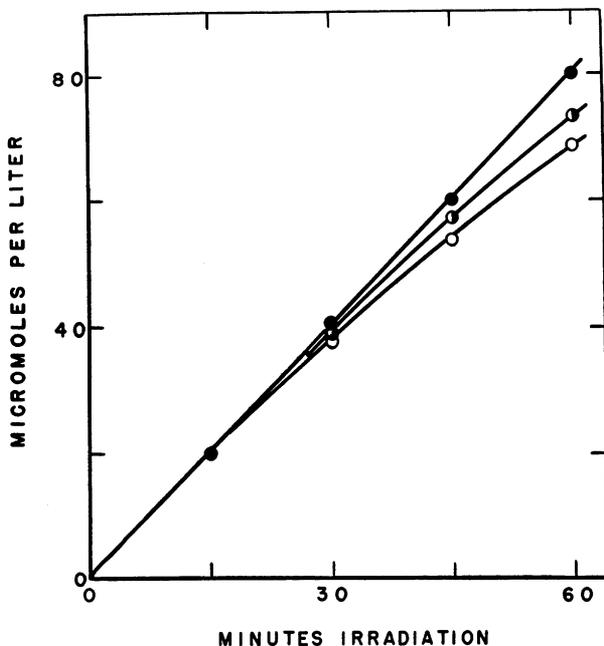
FIG. 7. Effect of benzene concentration on rate of production of phenol in radiolysis of aerated aqueous solutions of benzene in 0.8 N sulfuric acid. PhOH concentrations at different doses. Dose rate:  $3.03 \times 10^{19}$  ev/liter-min. Legend: ● saturated benzene solution; ● 50% saturated benzene solution; ○ 10% saturated benzene solution. Yields:  $G_0(\text{PhOH}) = 2.64$  for all benzene concentrations employed.
