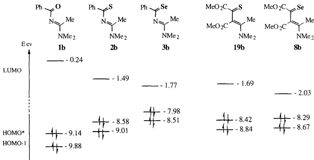
Figure 4 : Frontier Molecular Orbital energy levels by PM3 calculation ; \* Lone pair
