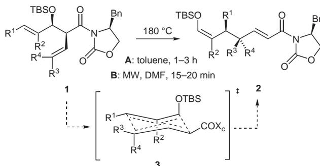
**Scheme 1** Cope rearrangement of aldol products **1** under standard (A) and microwave (B) conditions.
