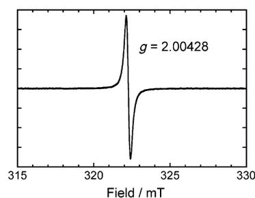
Figure 5. ESR spectrum of the anionic radical of TANC at room temperature under aerobic conditions.
