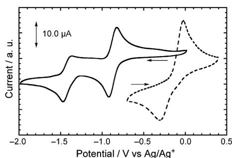
Figure 4. Cyclic voltammograms of **1a** (solid line) and **2a** (dashed line) at 1.0 mM in CH<sub>2</sub>Cl<sub>2</sub> (**1a**) and DMF (**2a**) solutions of *n*Bu<sub>4</sub>NPF<sub>6</sub> (0.10 M), at a scanning velocity of 100 mV s<sup>-1</sup>.
