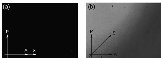
Figure 3. Polarized optical photomicrographs of the uniaxially aligned **1a** in the hexagonal columnar phase at room temperature by mechanical shearing. Rotating the sample by 45° gives periodic dark (a) and bright (b) images under the crossed Nicols condition. Arrows indicate the directions of the mechanical shearing (S), polarizer (P), and analysis (A) axes.
