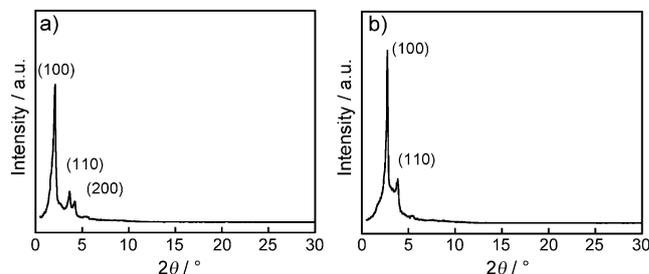
Figure 2. X-ray diffraction patterns of two LC states at room temperature: (a) **1a** in the hexagonal columnar structure and (b) **2a** in the tetragonal columnar structure.
