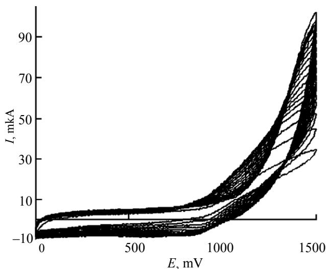
**Fig. 2.** Cyclic voltammogram of chalcone **X**, ITO-electrode, 20 cycles, Et<sub>4</sub>NClO<sub>4</sub>,  $V_{\text{scan}}$  50 mV s<sup>-1</sup>, CH<sub>3</sub>CN-CH<sub>2</sub>Cl<sub>2</sub>, 9 : 1.
