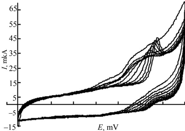
**Fig. 1.** Cyclic voltammogram of chalcone **X**, C-Si-electrode, 10 cycles, Et<sub>4</sub>NClO<sub>4</sub>,  $V_{\text{scan}}$  50 mV s<sup>-1</sup>, CH<sub>3</sub>CN-CH<sub>2</sub>Cl<sub>2</sub>, 9 : 1.
