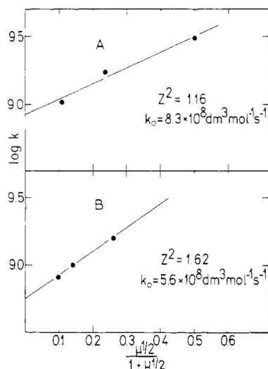
**Figure 1.** Ionic-strength dependence of the rate of oxidation of uric acid studied by pulse radiolysis of aqueous solutions at 5 Gy, 20 °C. (ionic strength was varied with KBr and KSCN): (A) oxidation of urate by  $\text{Br}_2^{\cdot-}$  at pH 7, and (B) oxidation of urate by  $(\text{SCN})_2^{\cdot-}$  at pH 11.16.
