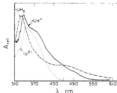
**Figure 2.** The absorption spectra of different forms of the urate radical obtained in  $\text{N}_2$  saturated aqueous solutions of  $0.1 \text{ mol dm}^{-3}$  KBr and  $1 \text{ mmol dm}^{-3}$  uric acid, at 20 °C, dose/pulse = 50 Gy: broken line, the neutral urate radical,  $\text{UH}_2^{\cdot-}$ , at pH 2; full line, urate radical anion,  $\text{UH}^{\cdot-}$ , at pH 7; and dotted line, double-deprotonated urate radical,  $\text{U}^{2\cdot-}$ , at pH 13.
