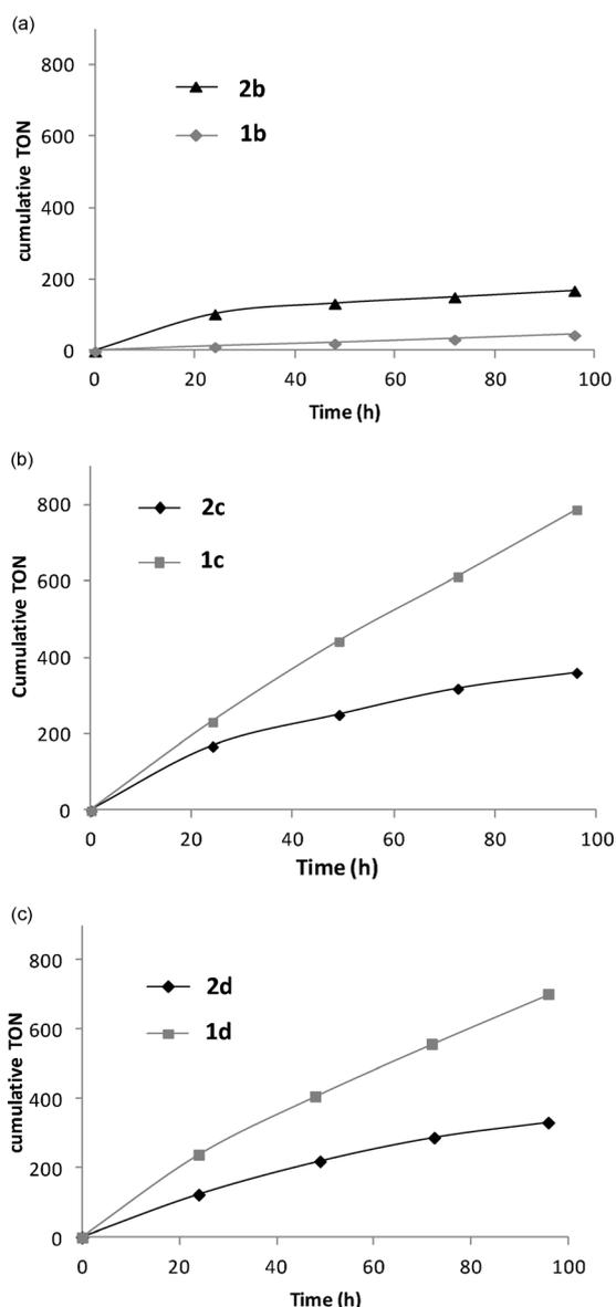
**Figure 3.** Influence of the architecture of the cavity on the catalytic reactivity of supramolecular azaphosphatranes **1b–d** and model analogues **2b–d**. Reaction conditions: styrene oxide (50.0 mmol), catalyst (0.05 mmol), CO<sub>2</sub> (1 bar), 100 °C. TONs were determined by <sup>1</sup>H NMR spectroscopy by using 2,4-dibromomesitylene (2.0 mmol) as an internal standard.
