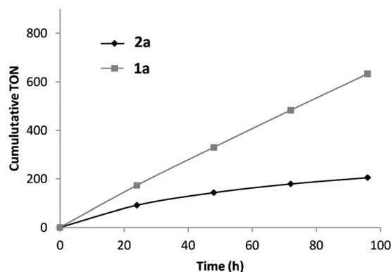
**Figure 2.** Effect of confinement on catalytic performances of supramolecular azaphosphatrane **1 a** and its model, **2 a**. Reaction conditions: styrene oxide (50.0 mmol), catalyst (0.05 mmol),  $\text{CO}_2$  (1 bar),  $100^\circ\text{C}$ . TONs were determined by  $^1\text{H}$  NMR spectroscopy by using 2,4-dibromomesitylene (2.0 mmol) as an internal standard.
