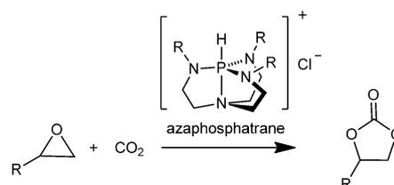
**Scheme 1.** Synthesis of cyclic carbonates from epoxides and carbon dioxide, catalyzed by azaphosphatranes.
