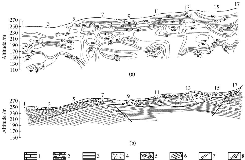
Fig. 6. Contour section of imitative resistivities (in  $\Omega m$ ) (a) and deduced geological section (b) for survey line  $E_4$ . 1, Limestone; 2, argillaceous limestone; 3, purplish-red mudstone; 4, soil and fine debris; 5, soil and coarse debris; 6, sliding mass; 7, sliding between layers; 8, sliding plane.
