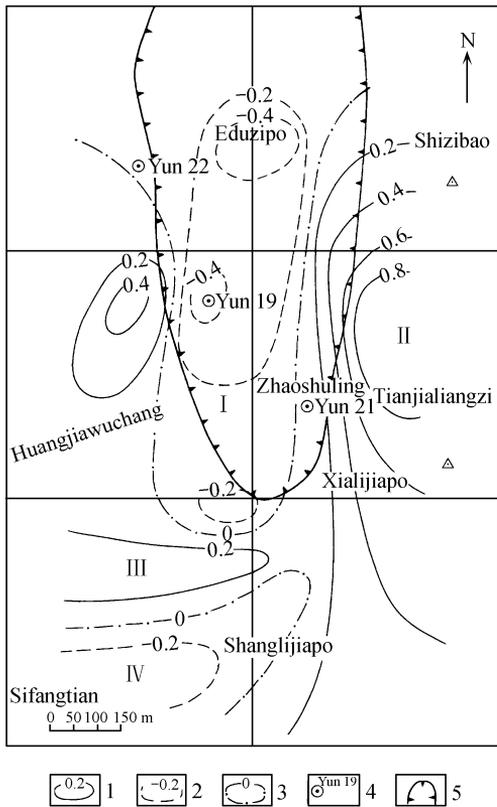
Fig. 8. Contour map of soil temperature anomalies (in °C) in study area. 1, Positive contour; 2, negative contour; 3, contour with zero value; 4, borehole and its number; 5, landslide boundary deduced by VSP, SRS, ES surveys.
