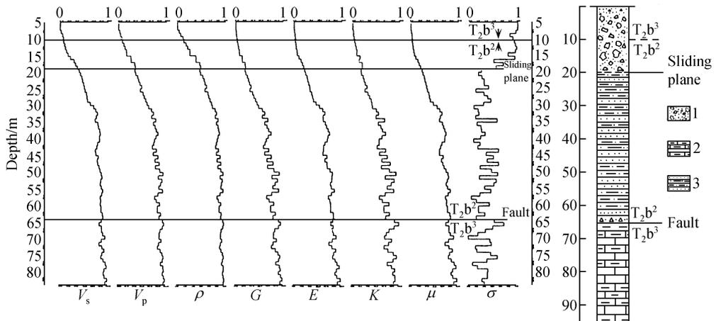
Fig. 4. Normalized electrodynamic modulus diagrams and borehole geological section in borehole Yun 19.  $V_s$ , Velocities of S waves;  $V_p$ , velocities of P waves. 1, Q; 2, argillaceous limestone, limestone interbedded; 3, argillaceous siltstone, sandstone interbedded.
