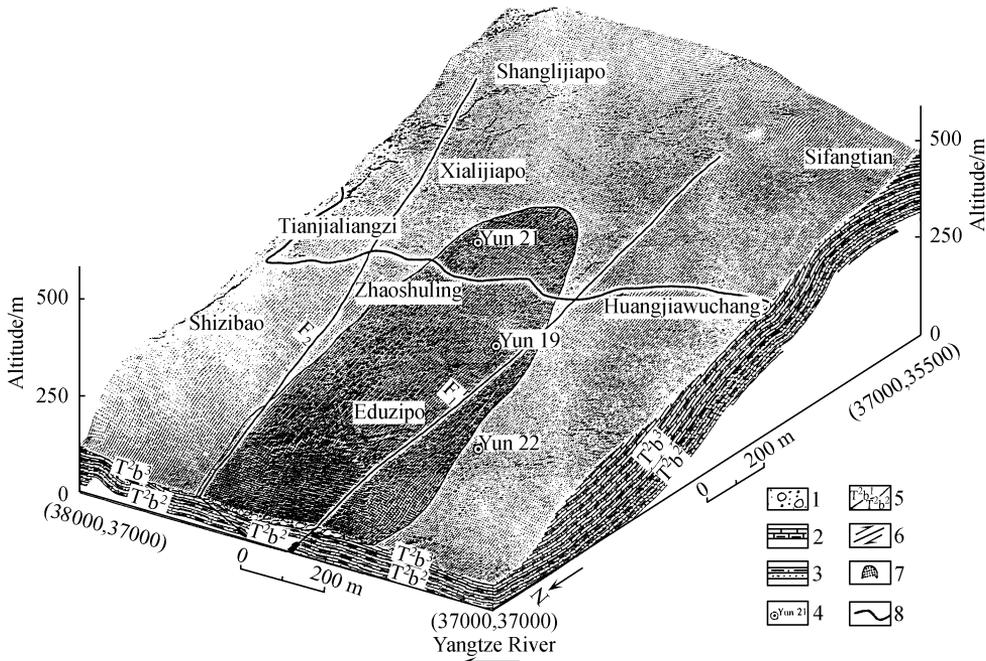
Fig. 7. Three-dimensional geological map of Zhaoshuling Landslide. 1, Q; 2, argillaceous limestone, limestone interbedded; 3, argillaceous siltstone, sandstone interbedded; 4, borehole and its number; 5, formation boundary; 6, reversed fault deduced by integrated geophysical survey; 7, limit of landslide; 8, simply-built highway.
