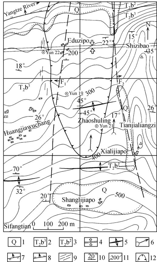
Fig. 1. Geological map of the study area. 1, Q; 2,  $T_2b^3$ ; 3,  $T_2b^2$ ; 4, axial trace of syncline; 5, axial trace of anticline; 6, small fold hinge; 7, reversed fault deduced by geophysical survey and its name; 8, normal fault; 9, reversed fracture zone; 10, occurrence; 11, formation boundary; 12, landslide boundary deduced by VSP, SRS and ES surveys.
