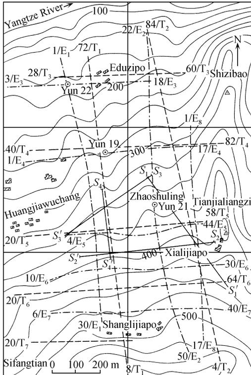
Fig. 2. Layout of geophysical survey.  $\odot$ , Yun 19: borehole and its number for VSP survey;  $S_1$ - $S_4$ ' , SRS survey line and its number;  $- \cdot - \cdot -$ , ES survey line;  $1/E_1$ , station number/line number for ES survey;  $- - -$ , ST and RG survey line;  $8/T_1$ , station number/line number for ST and RG survey.
