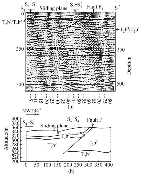
Fig. 5. SRS profile (a) and deduced lithologic and structural geological section (b) for survey line  $S_3-S_3'$ .
