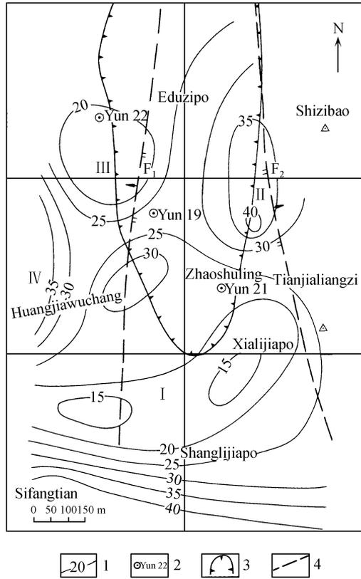
Fig. 9. Contour map of radioactive intensity of <sup>210</sup>Po (in pulse number/hour) in study area. 1, Positive contour; 2, borehole and its number; 3, landslide boundary deduced by VSP, SRS, ES, surveys; 4, reversed fault deduced by integrated geophysical survey.
