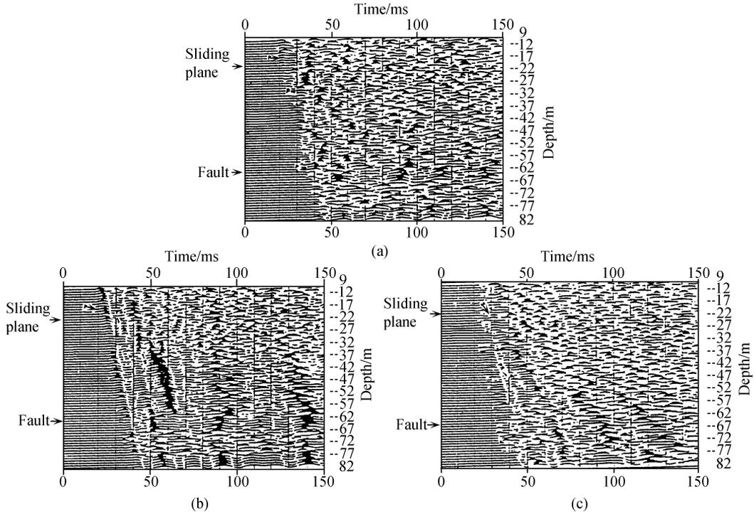
Fig. 3. Up-going wave profile (a), down-going wave profile (b) and shear wave profile (c) in borehole Yun 19.
