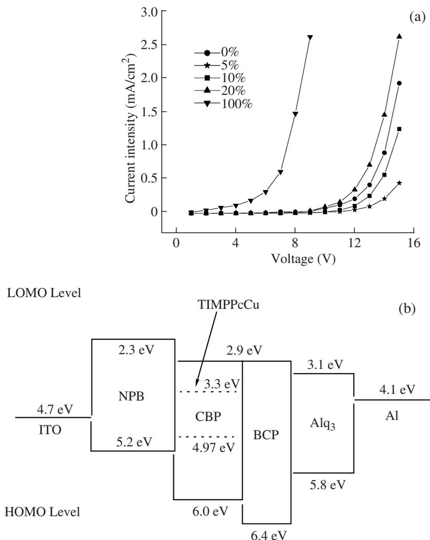
**Fig. 4.** (a) The current-voltage characteristics of OLEDs based on TIMPPcCu. (b) The energy level diagram of the devices containing TIMPPcCu.
