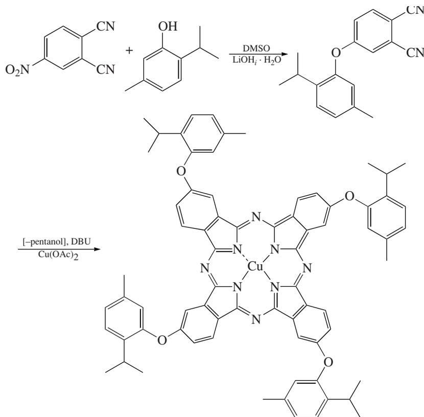
**Scheme 1.** The synthetic route of copper-tetra (2-isopropyl-5-methylphenoxy)phthalocyanine.
