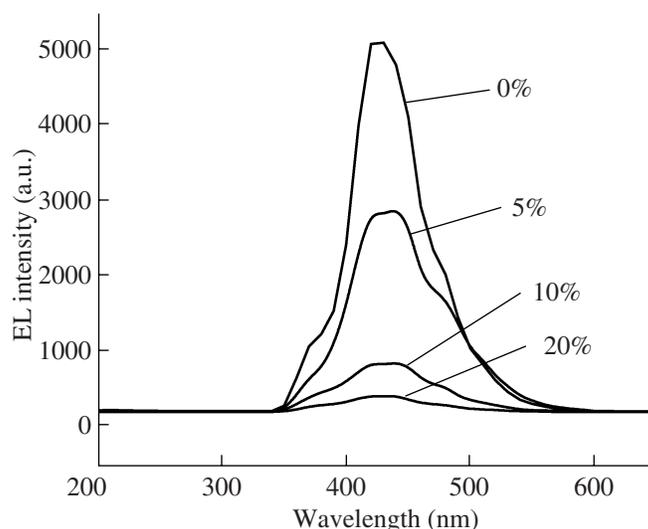
Fig. 3. The UV-vis EL spectrum of the doped OLEDs with different TIMPPcCu concentrations.
