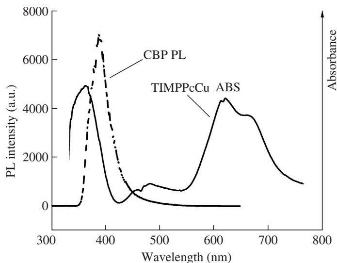
**Fig. 1.** The absorption spectrum of TIMPPcCu film and PL spectrum of CBP at room temperature (excited using 325 nm line from a He–Cd laser).
