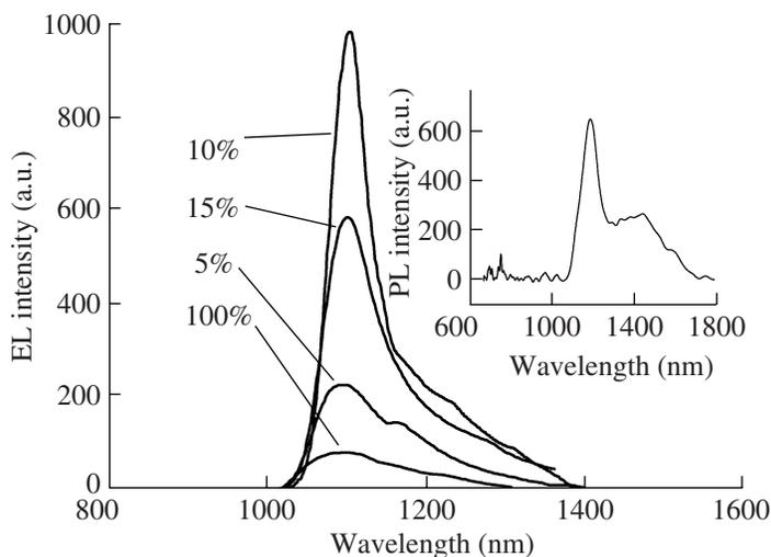
**Fig. 2.** The NIR EL spectra of devices based on TIMPPcCu with different concentrations in CBP (measured under the same conditions). Inset: The PL spectra of TIMPPcCu tablet excited using the 488 nm line from an  $\text{Ar}^+$  laser at 10 K temperature.
