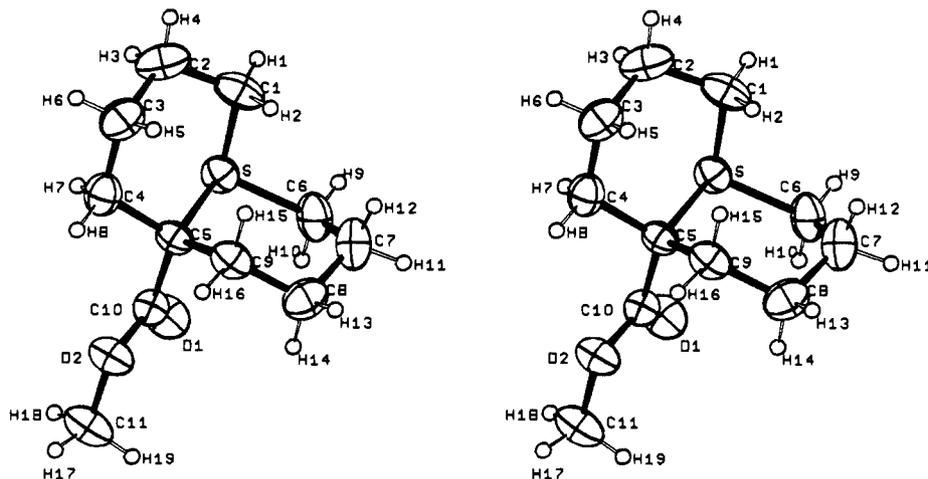
Figure 1. Stereodrawing (ORTEP) of the bicyclic sulfonium cation **9**. Hydrogen atoms are drawn with fictitious spherical thermal parameters of 0.5 Å<sup>2</sup>.
