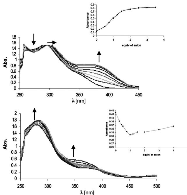
Figure 4. UV titration of ligand  $\mathbf{1}$  plus TBA oxalate (top) and ligand  $\mathbf{2}$  plus TBA oxalate (bottom) both in DMSO ( $3 \times 10^{-4}$  M, increasing addition until 4 equiv. at 25 °C). For the other anions studied, see the Supporting Information.
