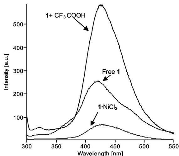
Figure 3. UV spectra of free, protonated (6 h after protonation) and Ni<sup>2+</sup>-complexed ligand **1** (top); fluorescence spectra of free, protonated (immediately after protonation) and Ni<sup>2+</sup>-complexed ligand **1** (bottom).
