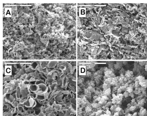
Figure 4. SEM images of polyethylene samples produced with complexes **6** (A) and **9** (B) and with the reference complexes  $\text{FeCl}_2(\text{Pr}^i\text{pdi})$  (C) and  $\text{CoCl}_2(\text{Pr}^i\text{pdi})$  (D). The bar scale represents 5  $\mu\text{m}$ .
