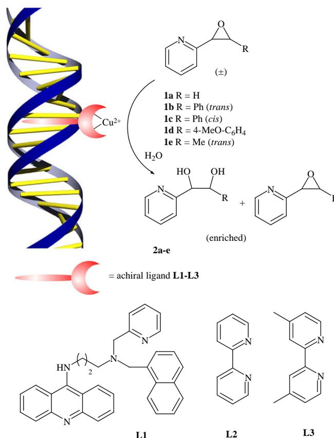
**Figure 1.** Schematic representation of the DNA-based hydrolytic kinetic resolution of 2-pyridyloxiranes **1a-e**.
