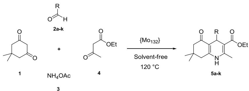
**Scheme 1.** Synthesis of polyhydroquinolines catalyzed by {Mo<sub>132</sub>}
