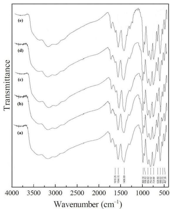
**Figure 3.** FT-IR spectra of fresh catalyst {Mo<sub>132</sub>} (a, first run), and recovered catalysts (b-e, second to fifth run, respectively) for synthesis of compound **5d** in model reaction.
