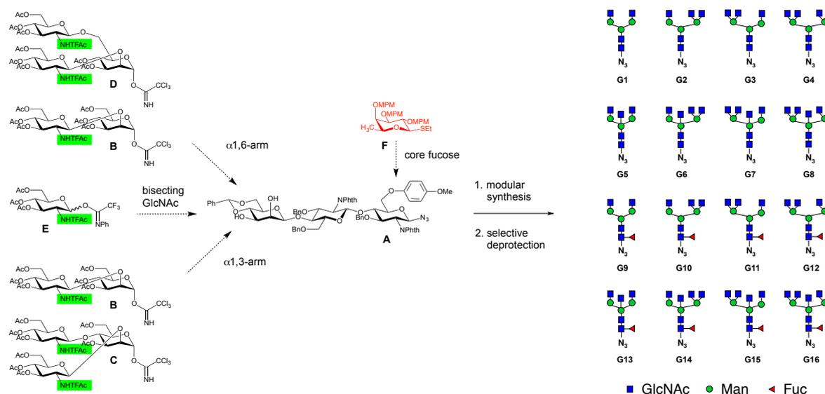
**Scheme 1:** Modular set of building blocks designed for the envisioned all-in-one-route to mammalian complex N-glycans **G1-G16** with optional bisecting GlcNAc and core fucose. Bn=benzyl, NPhth=phthalimido, Ac=acetyl, TFAc=trifluoroacetyl, MPM=p-methoxybenzyl, MP=p-methoxyphenyl.
