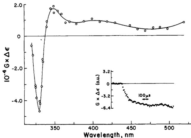
**Figure 5.** Difference absorption spectrum of  $C_{60}^-/\gamma$ -CD recorded 260  $\mu$ s after pulse radiolysis of aqueous solution of  $1.2 \times 10^{-5}$  mol  $dm^{-3}$   $C_{60}$ ,  $8 \times 10^{-3}$  mol  $dm^{-3}$   $\gamma$ -CD, and 0.1 mol  $dm^{-3}$  propan-2-ol saturated with nitrogen. Dose 2.3 Gy/pulse. Insert: Digitized traces of signal at 330 nm.
