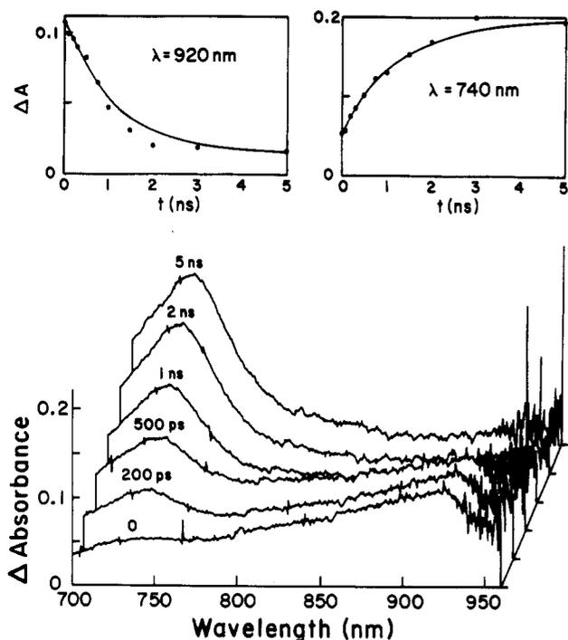
**Figure 1.** Time-resolved difference absorption spectra of singlet and triplet excited states of  $C_{60}/\gamma\text{-CD}$  in aqueous solution. Spectra were recorded following 355-nm laser pulse (pulse width 18 ps) excitation of  $1 \times 10^{-5} \text{ mol dm}^{-3} C_{60}$  and  $8 \times 10^{-3} \text{ mol dm}^{-3} \gamma\text{-CD}$ . Inserts show the decay of singlet (920 nm) and the formation of triplet (740 nm) excited states.
