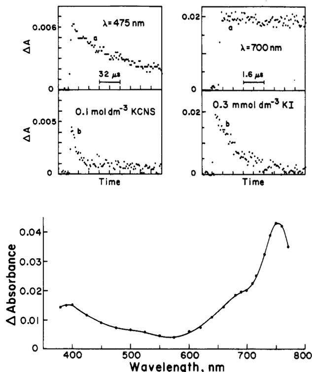
**Figure 2.** Difference absorption spectrum of triplet  ${}^3C_{60}/\gamma\text{-CD}$  in aqueous solution recorded after 337.1-nm nanosecond laser pulse excitation of  $6 \times 10^{-6} \text{ mol dm}^{-3} C_{60}$  and  $5 \times 10^{-3} \text{ mol dm}^{-3} \gamma\text{-CD}$ . Inserts show the time profiles of triplet signals (a) in the absence and (b) in the presence of anions.
