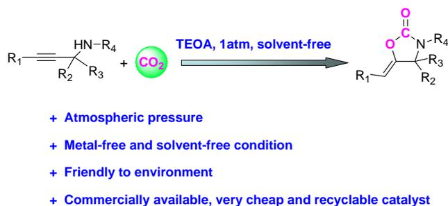
**Scheme 1.** Carboxylative cyclization of propargylic amines with CO<sub>2</sub> catalyzed by TEOA.
