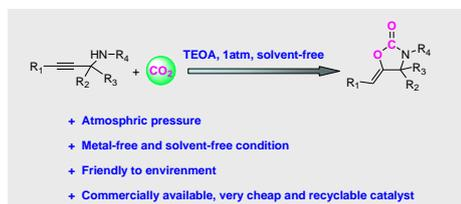
Triethanolamine (TEOA), as a low-cost and biodegradable catalyst, could efficiently promote the conversion of CO<sub>2</sub> with propargylic amine at atmospheric pressure.
