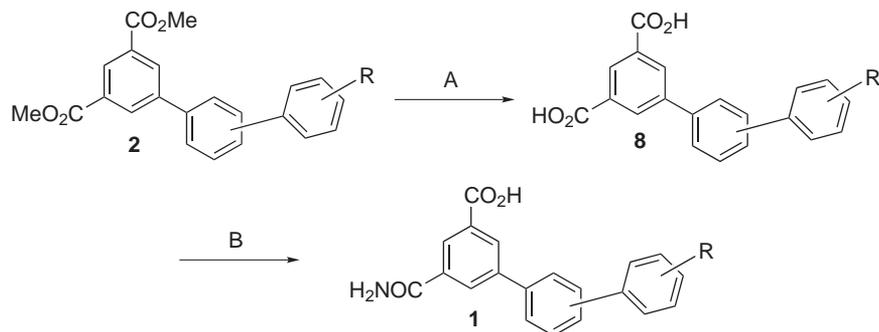
**Scheme 3.** (A) 0.1 M LiOH, THF; (B) (i) (COCl)<sub>2</sub>, cat. DMF, CH<sub>2</sub>Cl<sub>2</sub>, (ii) benzophenone imine, (iPr)<sub>2</sub>NEt, CH<sub>2</sub>Cl<sub>2</sub>, 0–5°C, (iii) 1N HCl, MeCN.
