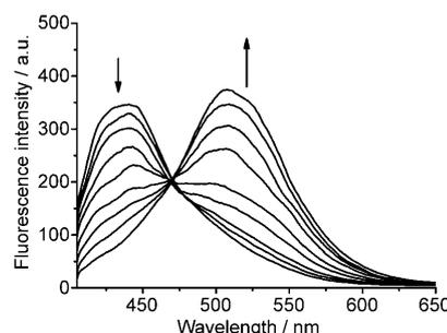
Figure 4. Fluorescence emission spectra of probe **1** (10  $\mu\text{M}$ ) in the presence of different concentrations of hypochlorite anion (0–30 equiv) in 0.1 M potassium phosphate buffer, pH 9.0/DMF (v/v, 1:4). Excitation wavelength was 394 nm.
