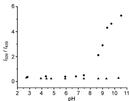
Figure 6. Ratios of the fluorescent emission intensities at 509 and 439 nm ( $I_{509}/I_{439}$ ) of probe **1** ( $10\ \mu\text{M}$ ) in the absence ( $\blacktriangle$ ) or presence ( $\bullet$ ) of  $\text{ClO}^-$  (30 equiv) at various pH values. Excitation wavelength was 394 nm.
