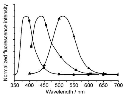
Figure 2. Normalized fluorescent emission spectra of compounds **1** (■), **2** (▲), and **3** (●) in 0.1 M potassium phosphate buffer, pH 9.0/DMF (v/v, 1:4), excited at 394, 394, and 326 nm, respectively.
