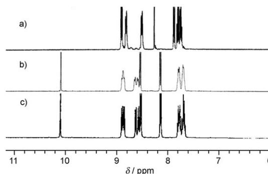
Figure 5. Partial  $^1\text{H}$  NMR (400 MHz) spectra of a) probe **1**, b) the separated product of probe **1** +  $\text{ClO}^-$ , and c) the standard compound **2**.
