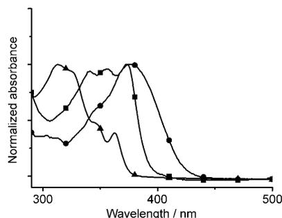
Figure 1. Normalized absorption spectra of compounds **1** (■), **2** (●), and **3** (▲) in 0.1 M potassium phosphate buffer, pH 9.0/DMF (v/v, 1:4).
