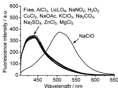
Figure 7. Fluorescence spectra of probe **1** ( $10\ \mu\text{M}$ ) in the absence and presence of 30 equiv of various species in 0.1 M potassium phosphate buffer, pH 9.0/DMF (v/v, 1:4). Excitation wavelength was 394 nm.
