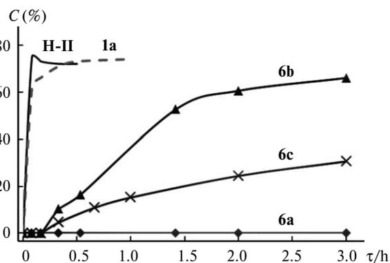
**Fig. 2.** Time dependency of allylbenzene conversion of a catalyst nature.
