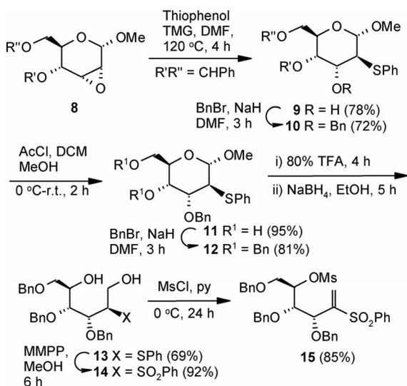
Scheme 3. Synthesis of hexosyl acyclic vinyl sulfone modified carbohydrates.
