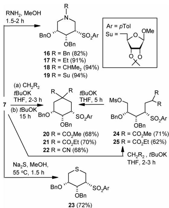
Scheme 4. Synthesis of six-membered heterocycles and carbocycles.
