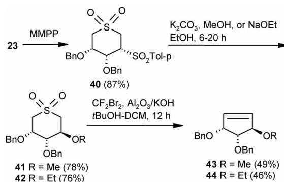
Scheme 7. Cyclopentenol derivatives from cyclic sulfide **23**.
