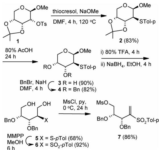
Scheme 2. Synthesis of pentosyl acyclic vinyl sulfone modified carbohydrates.
